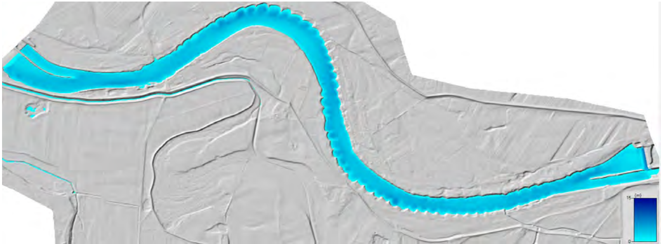
Fig. 2. Computed water depth along the study case river reach (TIN bathymetry) under Q_{276} flow conditions.
