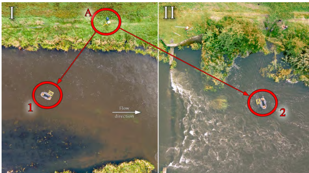
Fig. 1. Positions of the (A) precise total station, floating prism at the (1) upper and at the (2) lower position of the weir (UAV top-down photo).
